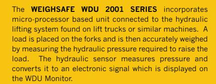
An accuracy of +/- 1 to 2% of the lift truck capacity is typically achieved. Designed for heavy industrial use, the lift truck can weigh a load in less that 5 seconds. This will ensure your shipments will not exceed trailer/truck capacity. Individual weight is displayed as a fixed reading, for up to 6 - 8 seconds when the "WEIGH" key is pressed, using the unique "Digi lock" software.
