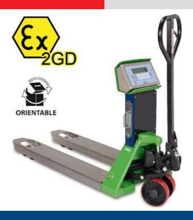
Pallet truck scales, with built-in electronic weighing, for dangerous areas classified as hazardous (ZONES 1 and 21 & 2 and 22) in accordance with Ex II 2G IIB T4 Gb X and Ex II 2D IIIC T197°C Db X.
