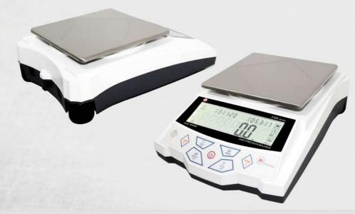
This is the Basic Precision balance 0,1g is the with the heavy duty design.
