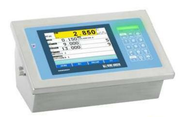
Weight indicator with a big touch screen display, for ATEX 2 & 22 areas classified at risk of explosion. Protection methods according to ATEX II 3G Ex nR IIB T6 Gc X for gases ATEX II 3D Ex tc IIIC T85°C Dc IP68 X for dust. Suitable for advanced industrial applications, it's fitted with 3 serial ports, configurable printouts and integrated alibi memory. CE-M approvable (OIML R-76 / EN 45501).
